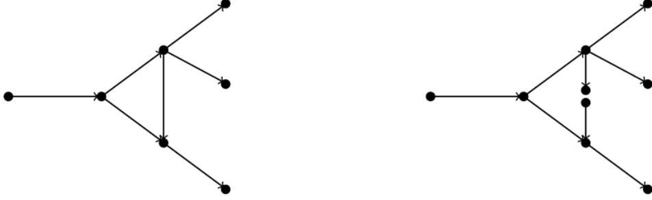
FIGURE 6. Construction of an auxiliary tree-shaped network (right) out of a network that contains a cycle (left) by adding one measurement point per cycle and cutting the cycle at this measurement point.
